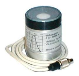
This type is meeting higher demands in accuracy. It's equpped with a light entrance window made of flat glass (or a PMMA dome if preferred). The material is UV-penetrable and long term resistant against radiation and environmental influences, and is therefore being used eg. in submarines and aircraft cockpits as well.
