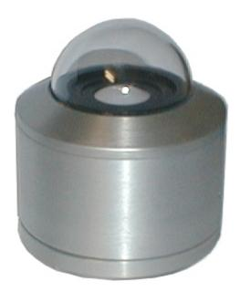
This type is meeting higher demands. It's equpped with a dome made of blown optical glass. This material is not UV-penetrable but long term resistant against radiation and environmental influences. The dome serves well as a light entrance window for radiation measuring devices. A few warpings due to the method of manufacturing only slightly increase the cosine error. Receiving characteristics are tested with great care.
